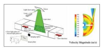
Figure 45. Test set-up for the performance evaluation of left heart simulator
