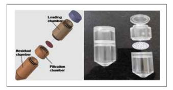
Figure 29. Design of the CTC filter (left) and the developed acrylic filter with different chambers (right)
