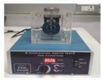
Catheter durability test setup for accelerated
